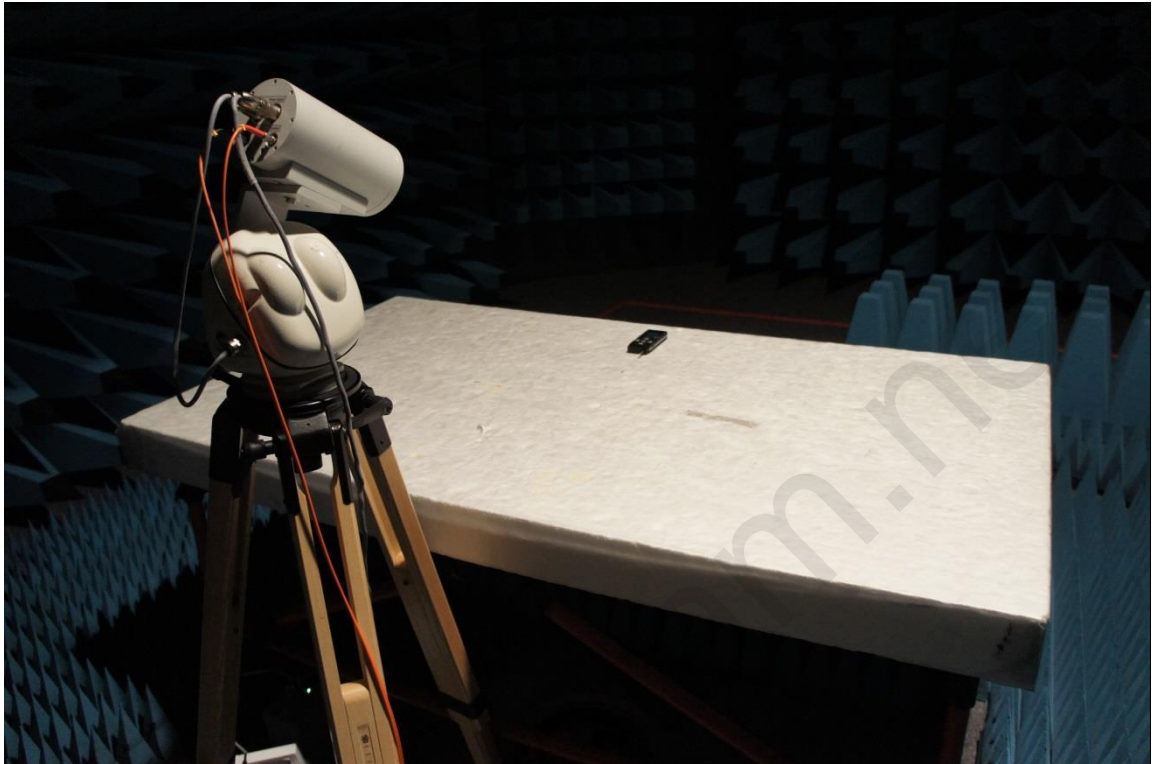
Picture 5: Test setup radiated immunity test
